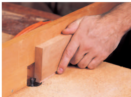
Figure 2: Rout tails on the rails with a dovetail bit and a router table, making sure the fit is just loose enough to slide them into the grooves in the sides.
