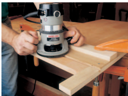
Figure 1: A T-square is ideal for routing the dovetail grooves. Make the jig using an extra wide piece of 1/4" plywood for the base, then trim it to size with your router and a 1/4" straight bit. Now you can align the edge of the base with your layouts and rout the grooves using a dovetail bit.
