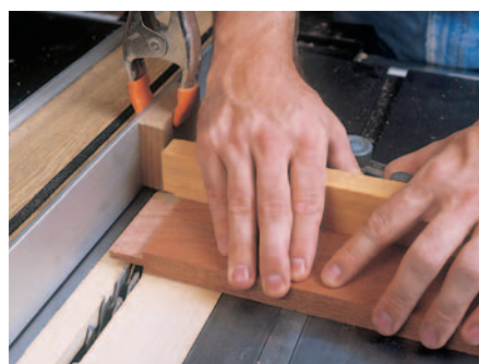
Figure 3: Clamp a set-up block to your fence to align the shoulder of your tenon layout with the \frac{1}{2} " dado blade. Make two passes to cut each cheek.
