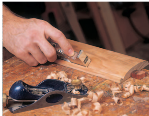
Figure 6: Trace the pattern of the top drawer face on the end of your stock and remove some of the waste with your table saw. Shape the face with a rabbet plane and block plane.
