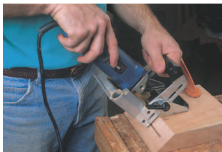
Figure 4: After mitering the front feet, cut slots with a biscuit joiner and join the pieces with biscuits. If you don't have a biscuit joiner, use splines.
