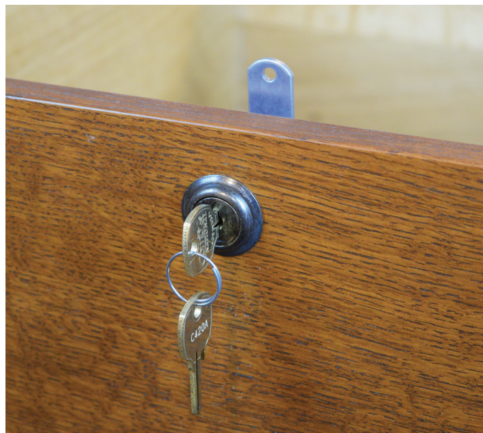
This photo shows the lock installation complete. The cam engages nicely with the biscuit slot, without interfering with drawer operation. Here, the cylinder lock is shown with optional trim ring installed (Antique Brass finish).
