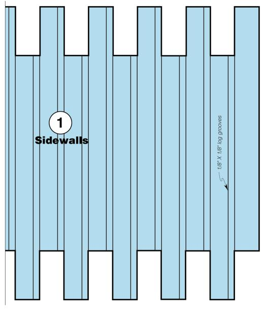
Lay out the notches, log-grooves, entry hole and gable ends from this pattern.
